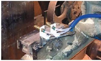
Band saw shown with two nozzles mounted just above guide and two additional nozzles mounted on the inside of the saw. Nozzles can be mounted any place on the inside back that is easy to attach. The objective is to coat the blade before it reaches the top wheel. This prevents pitch transfer to the wheel.
