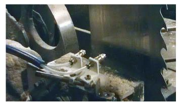
Front quide install on vertical mill saw
